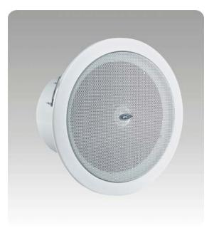
The built-in 4" full range high temperature resistant speaker driver is designed of wide frequency response 110-13kHz, the multiple power taps 3W & 6W are helpful for different applications varies from room size and ambient noise surroundings. The metal enclosure, aluminum grille with fire dom all are painted in attractive white color and a fire dome metal can is supplied. Its spring clamp makes the easy and secure installation.
